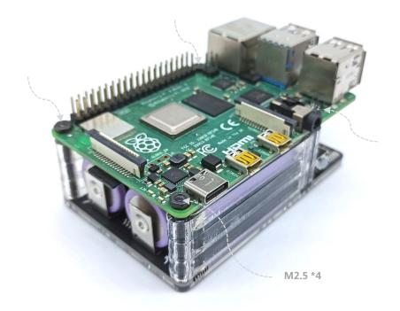
c. To remove and replace the battery, please use tweezers to insert it in the direction indicated by the arrow on the board and then pry up the battery
