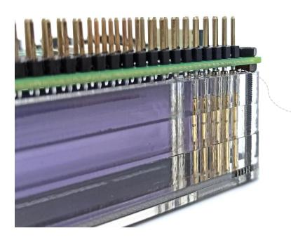
Make sure the pin header is aligned with the pogopin
